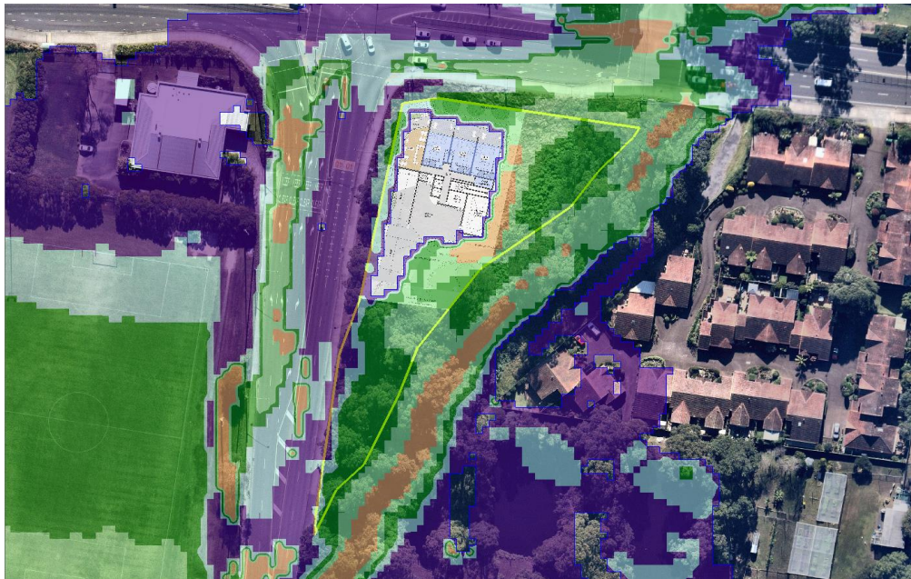
Figure 5.2-3 1% AEP Post-Development Flood Hazard
